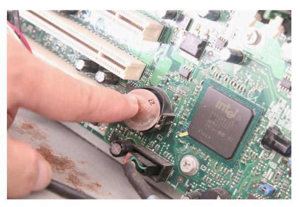
**4. Motherboard:** Remove the CMOS Battery and leave it out for about 15 seconds. Put the battery back in and then try to restart the computer.
