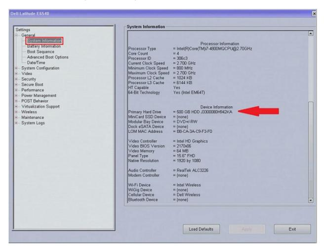
**1. BAD Hard Drive:** Make sure the hard drive is showing up. If not, the hard drive is bad ad need to be replaced.
