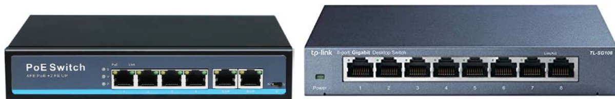
POE Switch and Network Switch
